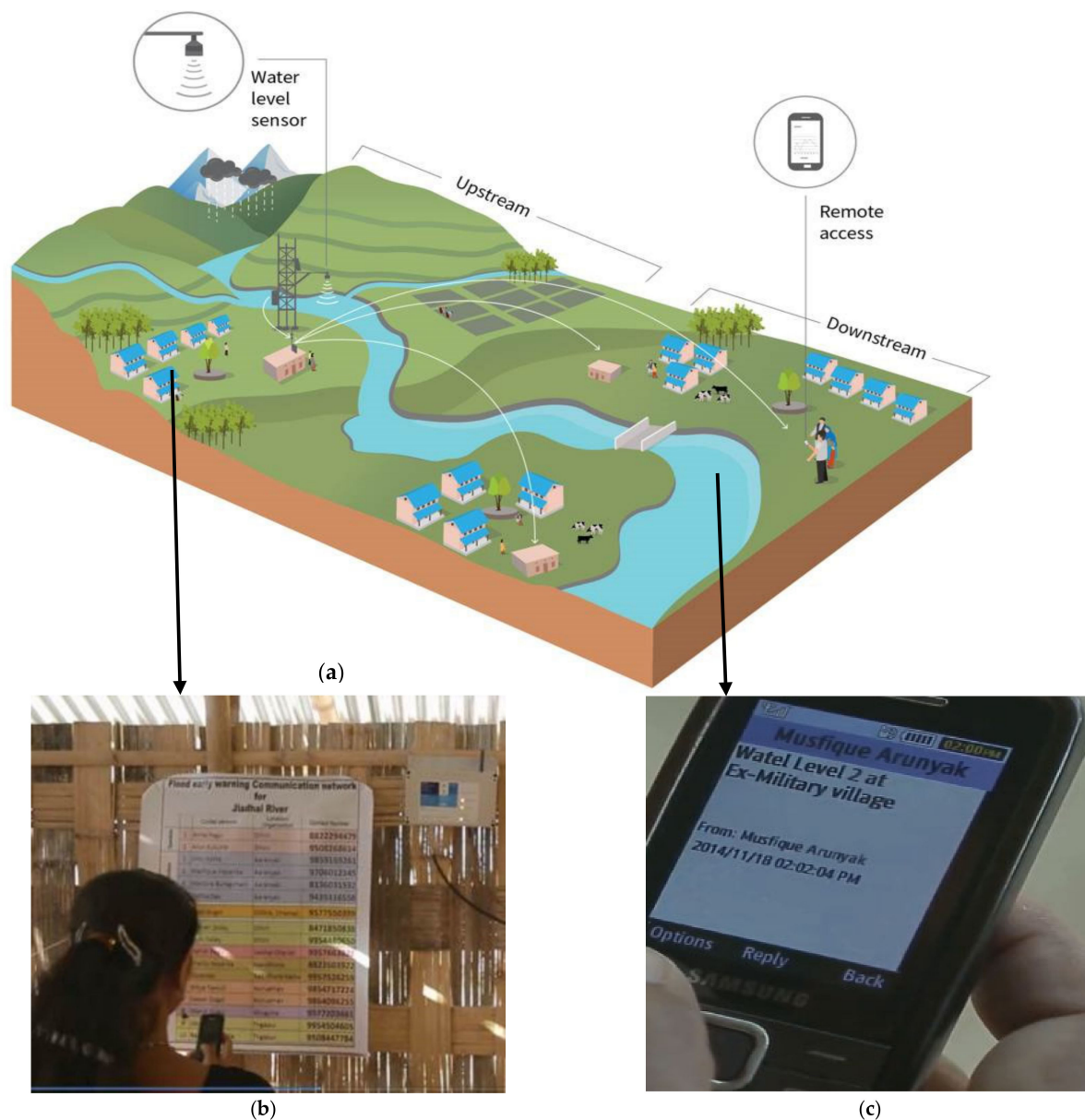
Figure 6. Schematic diagram of CBFEWS (a); caretaker monitoring receiver and dissemination flood information (b); and vulnerable communities receive warning information (c).
